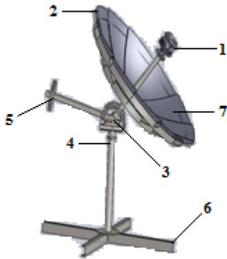
Fig. 10: Assembled drawing of the parabolic thermal cooker.
