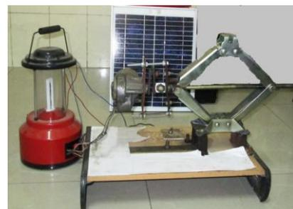
Fig. 1: Screw jack operated by solar battery
