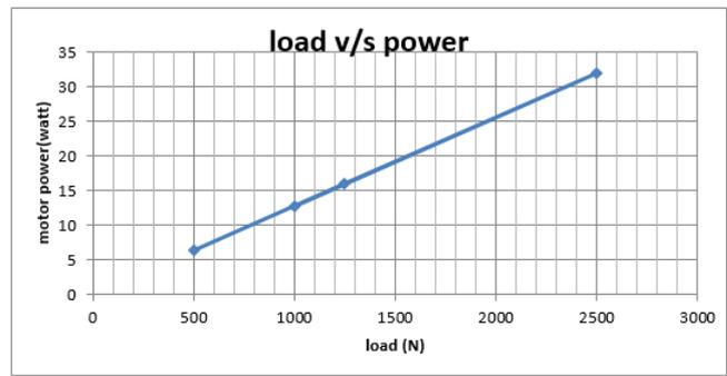
Fig. 4.3: Graph between load lifted and motor power
