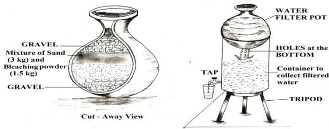
Fig: 1- Rooftop rain water harvesting 2-Percolation pits 3-chaals/ponds 4 - Slow Sand filtration 5- The pot chlorinator
