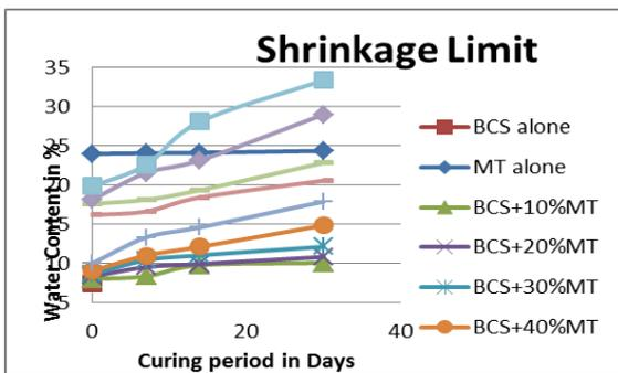
Fig. 8: Shrinkage Limit BC soil with Varying Percentages of mine tailings for Various Curing Periods
