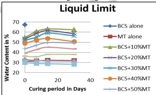
Fig. 4: Liquid Limit of BC soil with Varying Percentages of mine tailings for various Curing Periods
