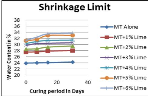
Fig. 2: Shrinkage Limit of mine tailings with Varying Percentage of Lime for various curing periods
