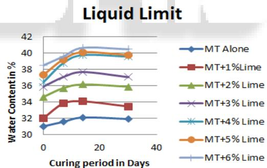
Fig. 1: Liquid Limit of Mine tailings with Varying Percentages of Lime for different Curing periods
