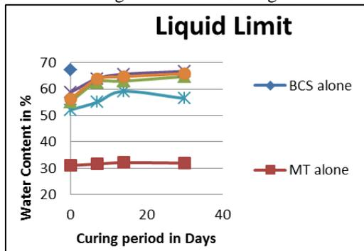
Fig. 5: Liquid Limit of BC soil with optimum percentage of mine tailings lime and sodium salts for various curing periods
