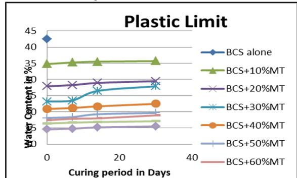
Fig. 6: Plastic Limit of BC soil with Varying Percentage of mine tailings for various curing periods
