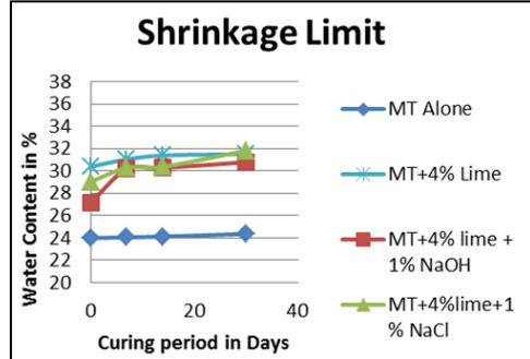
Fig. 3: Shrinkage limit of mine tailing with optimum percentage of lime and sodium salts for various curing periods
