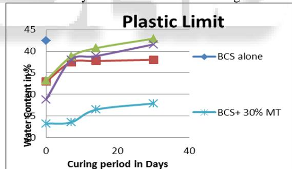
Fig. 7: Plastic limit of BC soil with optimum percentage of mine tailings-lime and sodium salts for various curing periods
