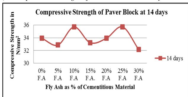
Fig. IX: (B) Compressive Strength of Paver Block at 14 Days
