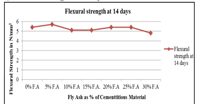
Fig. IX: (F) Flexural Strength of M-35 Mixes at 14 Days
