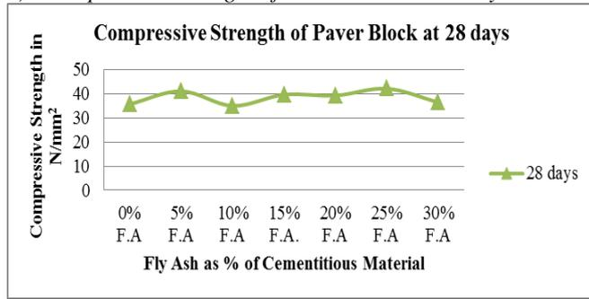
Fig. IX: (C) Compressive Strength of Paver Block at 28 Days
