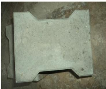
Fig. VIII: (D) Cross Section of Concrete Paver Block Specimens after Curing
