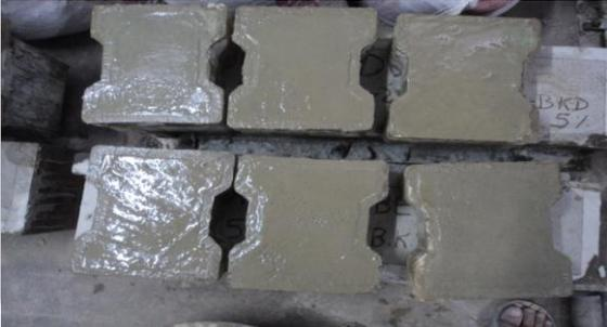
Fig. VIII: (C) Casting concrete Paver Blocks
