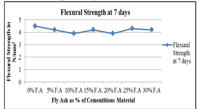
Fig. IX: (E) Flexural Strength of M-35 Mixes at 7 Days
