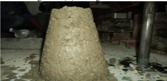
Fig. VIII: (B) Slump Test (Taken Sample Value = 0 mm)
