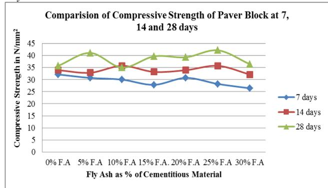
Fig. IX: (D) Compressive Strength of Paver Block at 7, 14 and 28 Days
