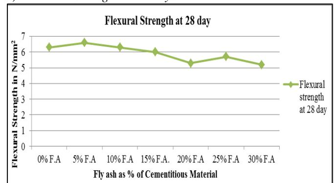
Fig. IX: (G) Flexural Strength of M-35 Mixes at 28 Days
