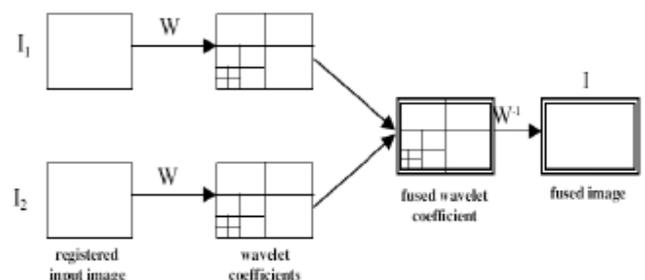
Fig. 4: Block Diagram Of DWT based Image Fusion[3]
