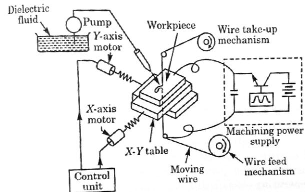
Fig. 1: Wire EDM model
