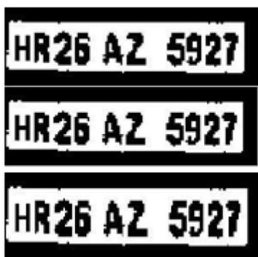
Fig. 8: Gnow image, Converted Black to white, connected component analysis
