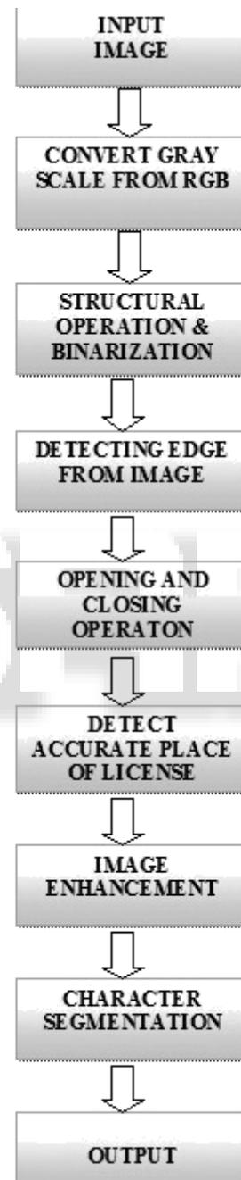
Fig. 1: Flowchart of SLPR Algorithm
