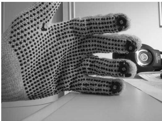
Fig. 1: Glove with Sensor
