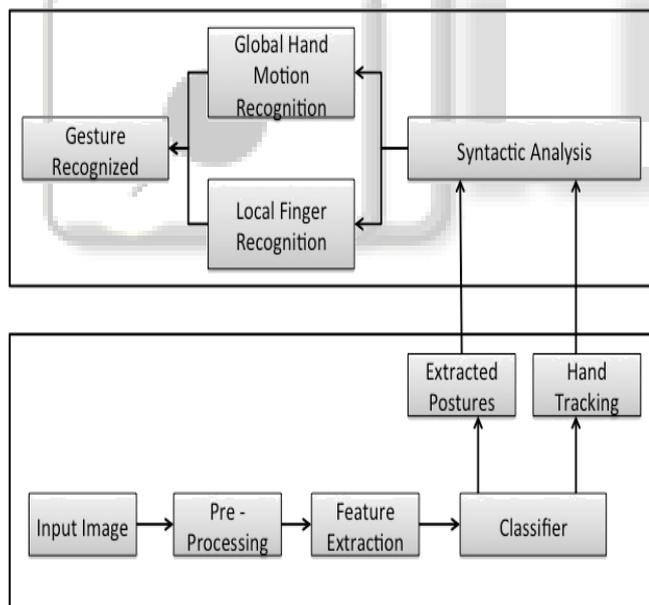
Fig. 5: Software Architecture
