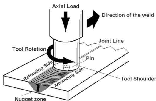
Fig. 1: Schematic Diagram of FSW
