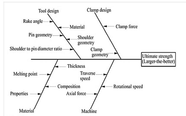
Fig. 2: Cause & effect Diagram of factors influencing Friction Stir Welded joint strength
