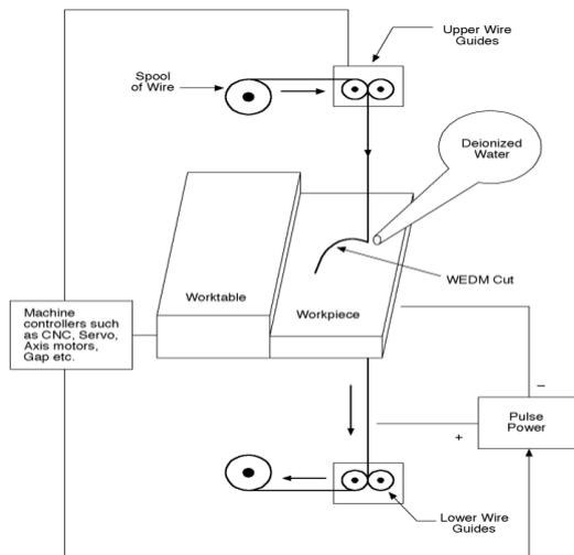
Fig. 1: Schematic Diagram of WEDM
