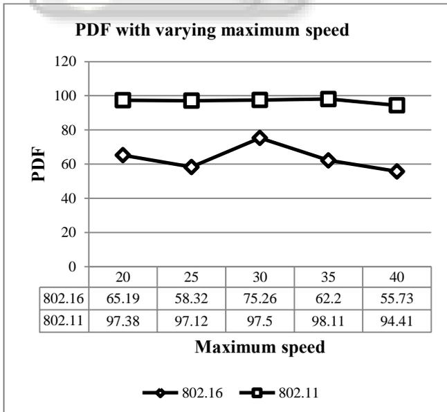
Fig. 1: Graph of PDR using On Demand Uncast Reactive Routing Protocol
