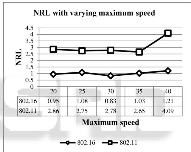
Fig. 3: Network Load for MAC layer control 802.11 and 802.16 using AODV
