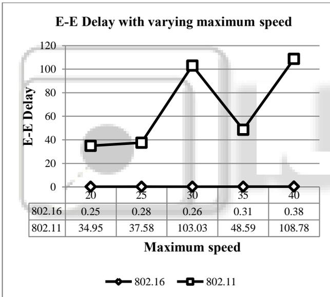
Fig. 6: E-E delay for MAC layer control 802.11 and 802.16 using DSR
