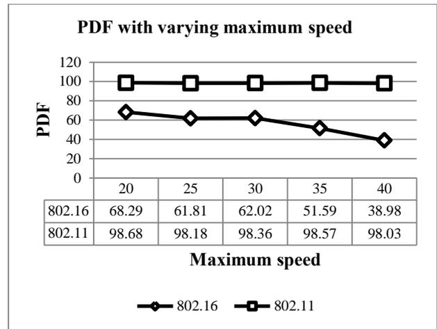
Fig. 2: Graph of PDR using On DSR Protocol
