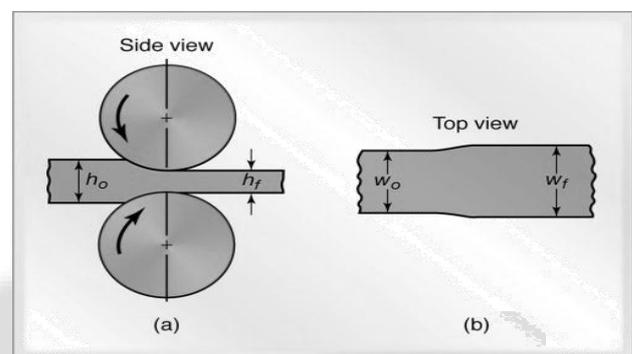
Fig. 1 (a) side view of metal passes through rolls (b) top view of metal stock
