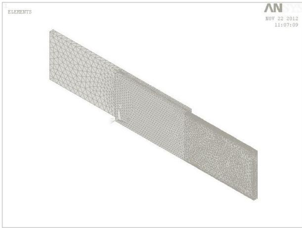
Fig. 10: Meshing Diagram Single Lap Joint
