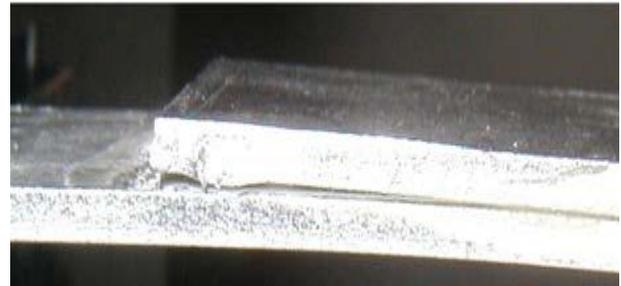
Fig. 8: Failure Mode Lap Joint
