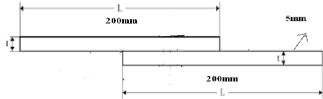
Fig. 4: dimension of Single Lap Joint
