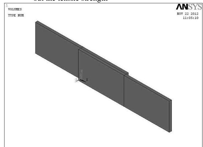
Fig. 9: Single Lap Joint
