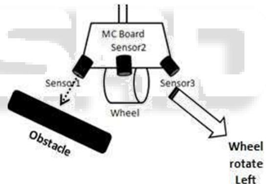
Fig. 4: Wheel rotating left for right side obstacle
