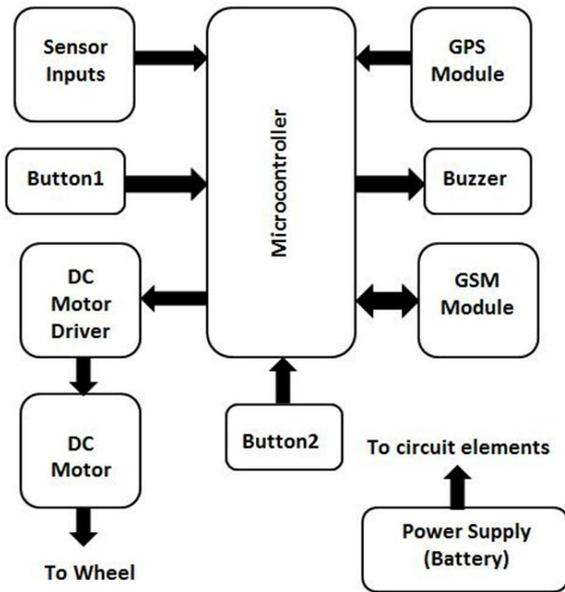
Fig. 2: Block diagram of microcontroller board elements
