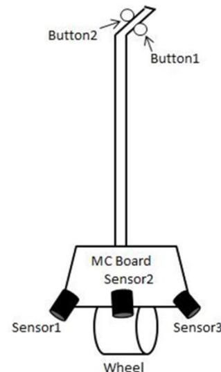
Fig. 1: Steering navigation stick for visionless person
