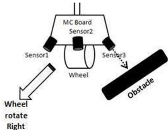
Fig. 5: Wheel rotating right for left side obstacle
