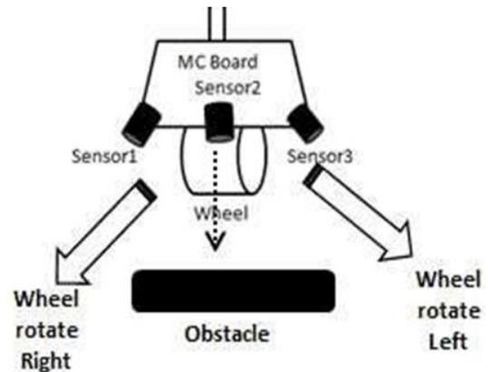
Fig. 3: Wheel rotating left/right for front obstacle
