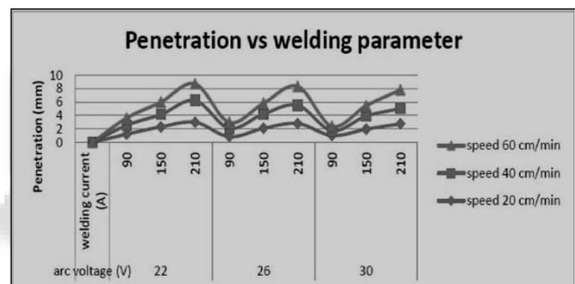
Fig. 3: Penetration vs. Welding Current & voltage
