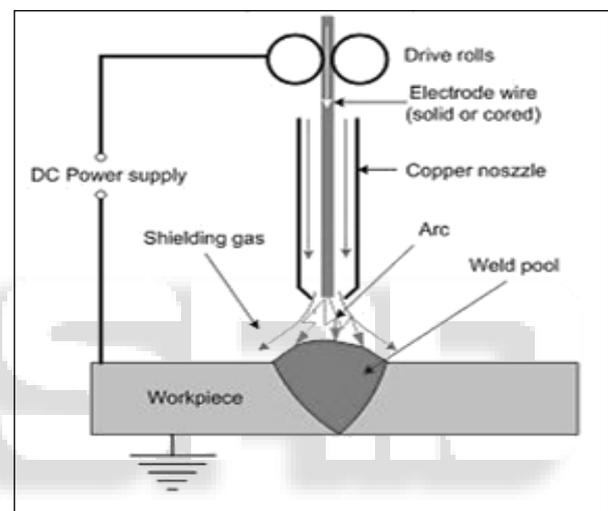
Fig. 1: Gas metal arc welding
