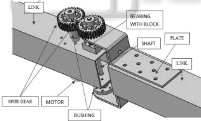
Fig. 5: joint between two Segments, CATIA model
