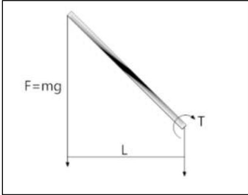
Fig. 4 Load acting on link
