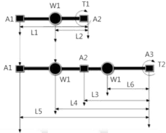
Fig. 7: Load and torque on joints
