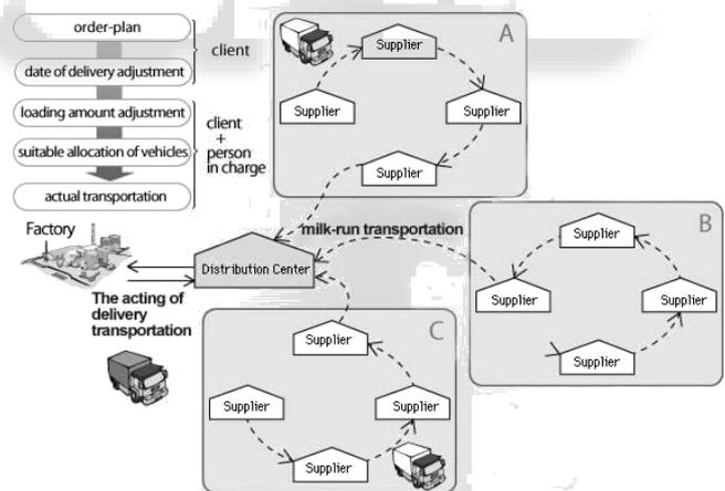
Fig. 2: Shows milk-run supply system for the manufacturing unit
