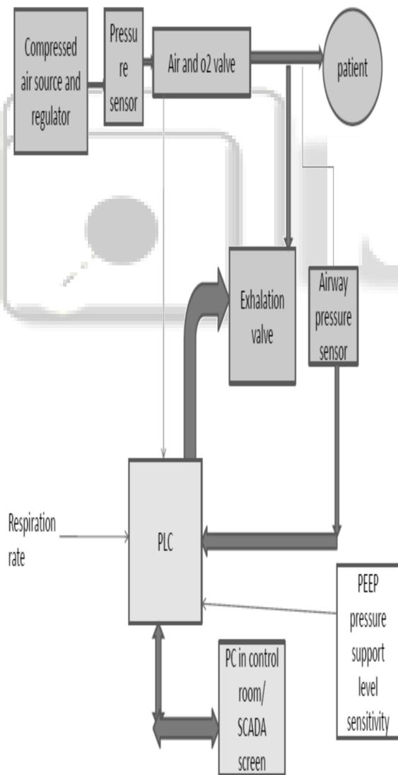
Fig. 3: Block diagram representing the various components required
