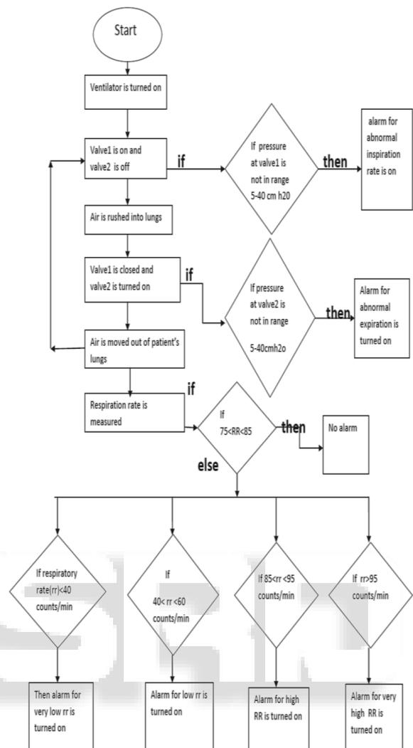
Fig. 4: Algorithm for the monitoring of ventilator for single patient
