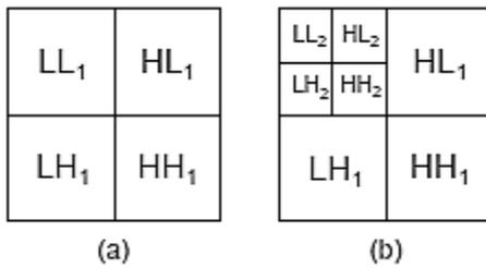
Fig. 1: 2D-DWT applied (a) once and (b) twice.
