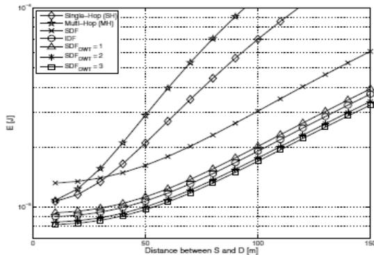
Fig. 2: Energy consumption in a NLOS scenario, for  $\mathcal{O}^* = 10^{-2}$  and  $\Delta = 2$  bits/s/Hz.
