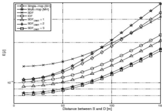
Fig. 3: Energy consumption in a LOS scenario, for  $\mathcal{O}^* = 10^{-2}$  and  $\Delta = 2$  bits/s/Hz.
