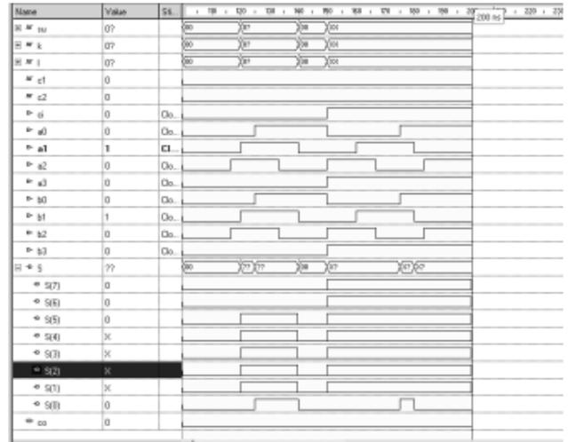
Fig. 9: Output for Hierarchical Multiplier
