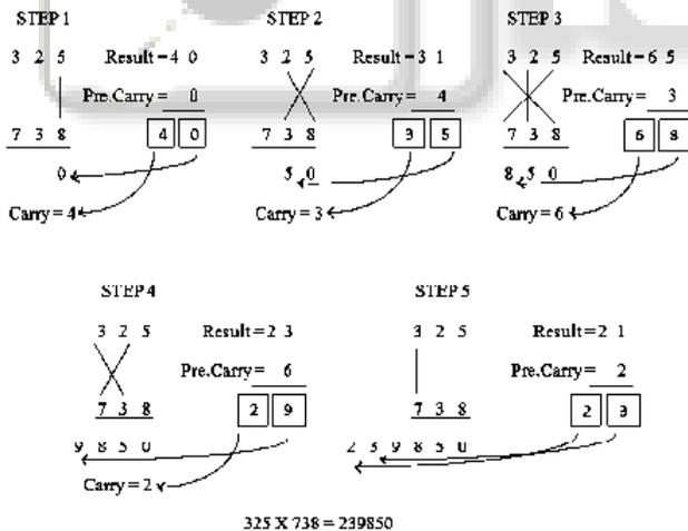
Fig. 2: Multiplication of two numbers using Urdhva Tiryakbhyam Sutra
