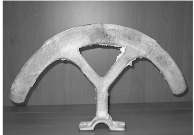
Fig. 2: Stainless steel shell casting component (Production part)
