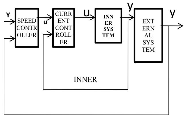
Fig. 3: Cascade control of the system
