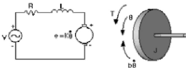
Fig. 1: Permanent magnet brushed dc motor
