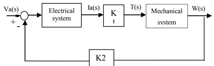
Fig. 2: DC motor block diagram
