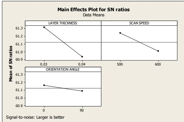
Fig. 4: Main Effect plot for SN Ratios (Tensile Strength)
