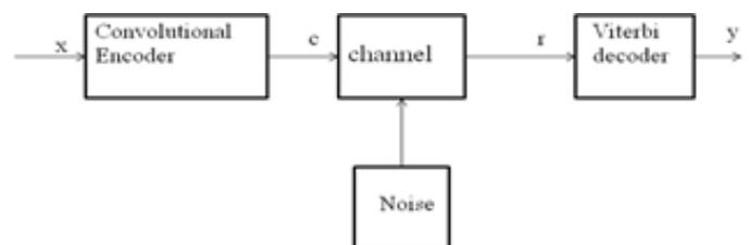
Fig. 1: Simple Viterbi decoder system
