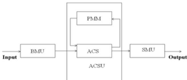
Fig. 3: Block Diagram of Viterbi decoder
