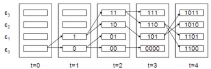
Fig. 4: Register Exchange Method
