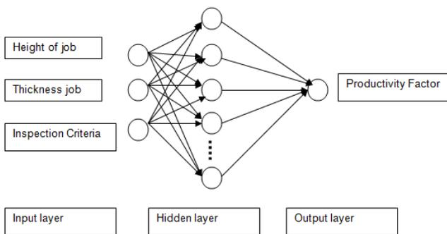
Fig. 1: Structure of the neural network
