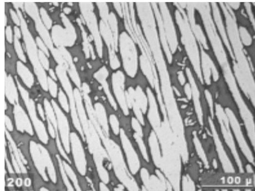
Fig. 5: DSS Micrograph at 200X
