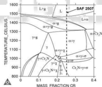
Fig 1. Phase diagram of SAF 2507 computed using the thermodynamic computer program Thermocalc. The composition of SAF 2507 is indicated by a dashed line.
