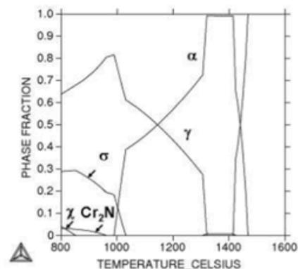
Fig 2. Phase fractions of ferrite, austenite,  $\sigma$ -phase,  $\chi$ -phase and Cr<sub>2</sub>N as a function of temperature in SAF 2507. Computed using Thermocalc.
