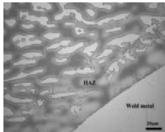
Fig 5: Weld 2-HAZ microstructure of cap bead.
