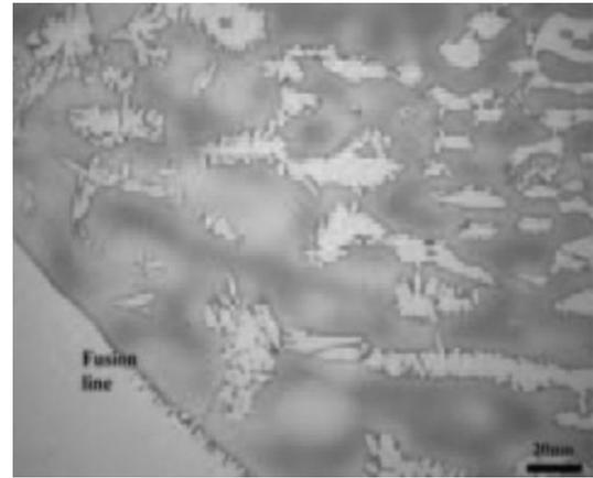
Fig. 4: Weld 1 - HAZ microstructure of cap bead.
