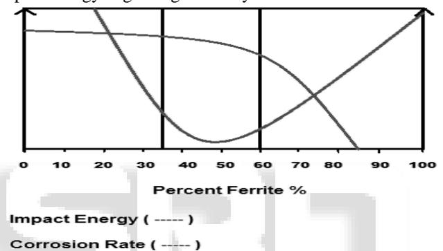
Fig. 3: Corrosion rate and impact energy vs. percent ferrite of DSS
