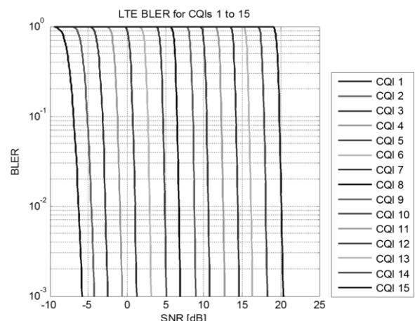
Fig. 3 BLER (Block Error Rate) for CQIs
