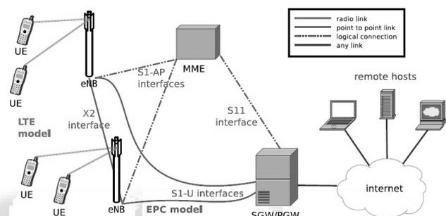
Fig. 1 Service Architecture Evolution in LTE network<sup>[1]</sup>
