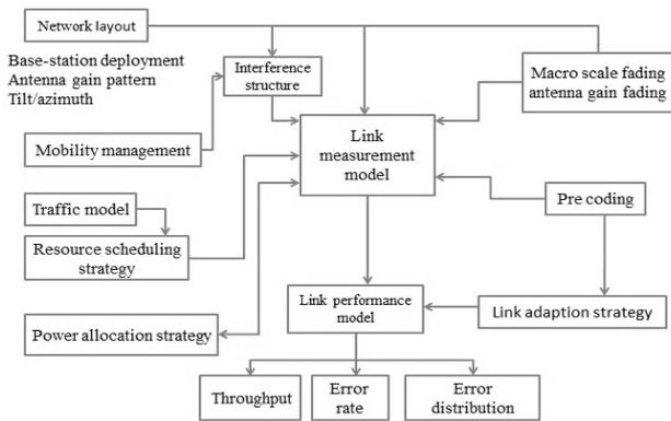
Fig. 2 LTE system level simulator
