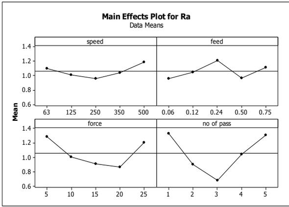
Fig. 7: Main effect plot for Surface roughness
