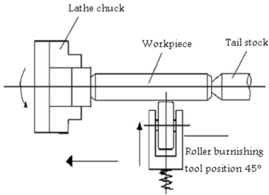
Fig. 2: Layout of work piece on lathe for roller burnishing process
