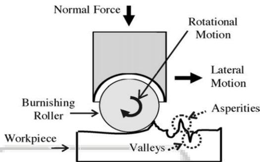
Fig. 3: Schematic Diagram of Basic Principle of Roller Burnishing Process
