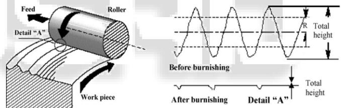
Fig. 1: roller burnishing process.
