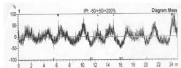
Fig 2. Mass diagram of wool yarn in 25 m.
