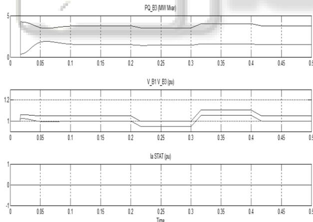
Fig. 4: Simulation Results without D Statcom
