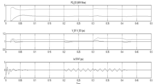
Fig. 5: Simulation Results with D- Statcom
