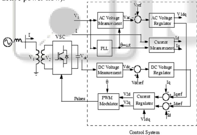
Fig. 1: control circuit of STATCOM
