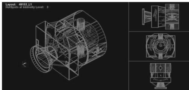
Fig. 4: Hot Spot Prediction at Level 3
