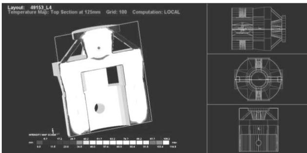
Fig. 6: Temperature Distribution of Modified Gating
