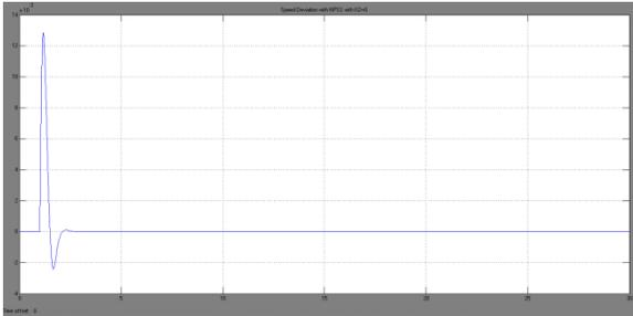
Fig. 12: Speed deviation versus time (NPSS)
