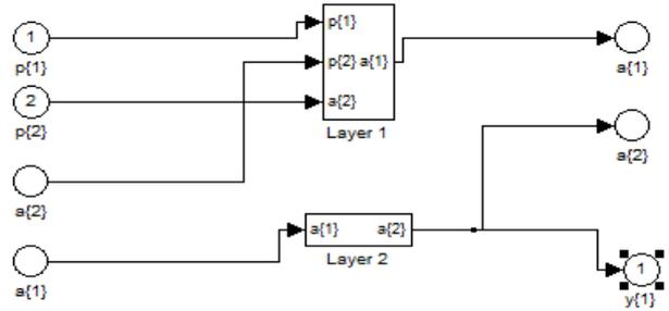
Fig. 7: Simulink block of neural network used as a Neuro-controller
