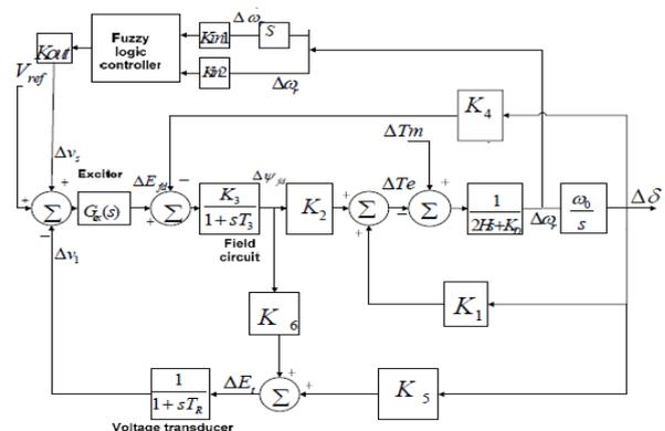
Fig. 4: Block diagram of fuzzy logic controller implemented on single machine infinite bus system
