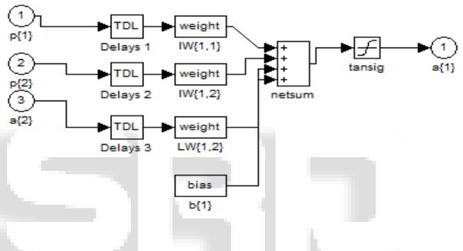
Fig. 8: Simulink block of input and hidden layer of Neuro-controller
