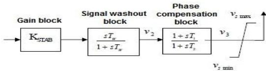
Fig. 3: Block Diagram of Conventional PSS
