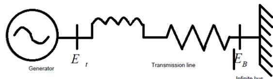
Fig.1: Synchronous Machine Connected To Infinite Bus
