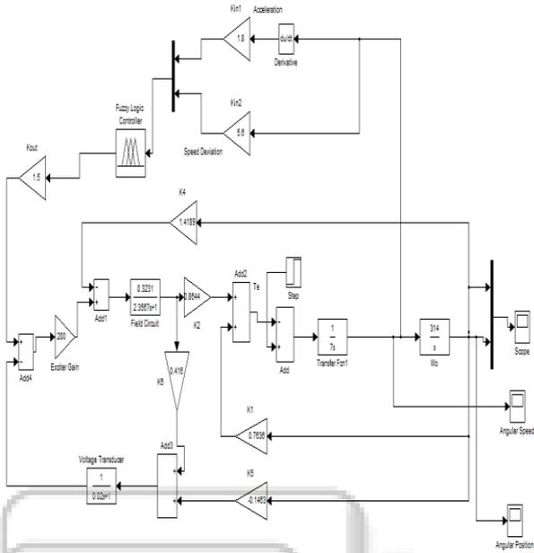
Fig. 5: Simulink model with Fuzzy Logic Based PSS
