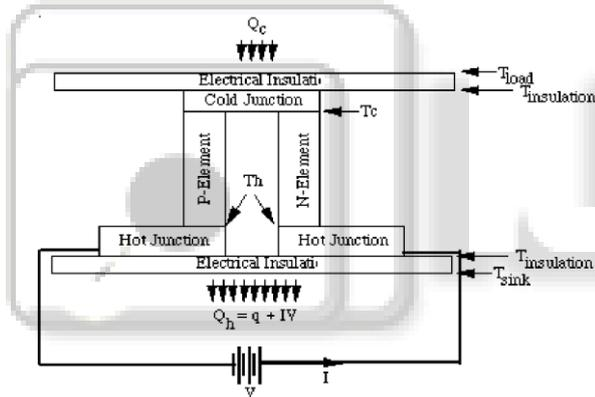
Fig. 6: Thermal network model of TER
