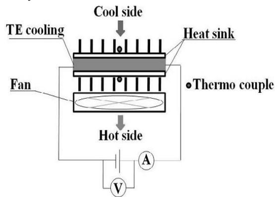
Fig. 3 : diagram for electric values measure
