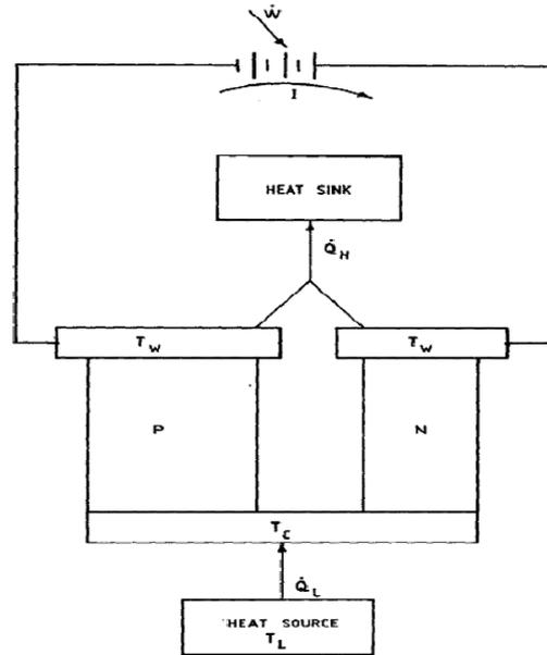
Fig. 2 A thermoelectric refrigerator
