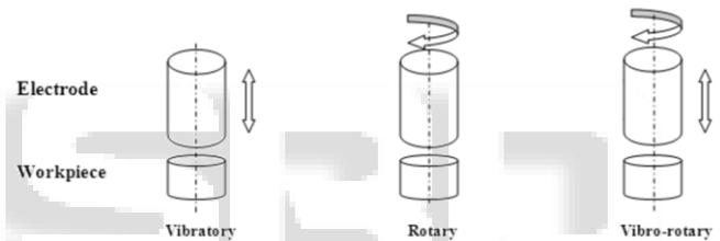
Fig. 2 : Vibratory, rotary and vibro-rotary electrode [6]
