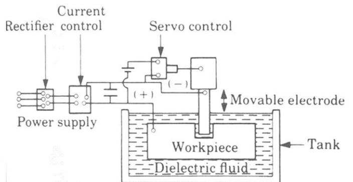
Fig: 1 Die-Sinker EDM Setup [1]
