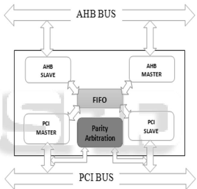
Fig. 2: PCI/AHB Bridge Component Architecture
