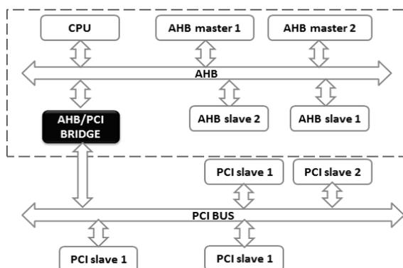
Fig. 1: PCI/AHB Bridge
