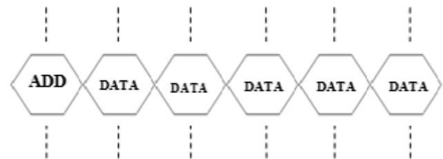
Fig. 3: PCI Burst Transfer
