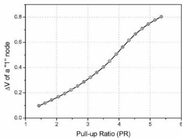
Fig 7: The voltage drop at node  $V_{v1}$  during write access as a function of the Pull-Up ratio (PR) ( $CR = \frac{W_4/L_4}{W_6/L_6} = \frac{W_5/L_5}{W_3/L_3}$  in Figure 2.3) of a 6T CMOS SRAM cell (simulated in CMOS 0.13 $\mu$ m technology,  $V_{DD}=1.2V$ ).
