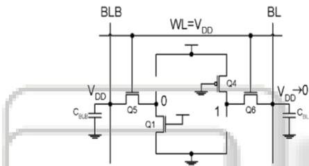
Figure 6 Simplified model of a 6T CMOS SRAM cell during a write operation
