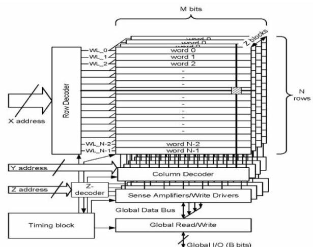
Fig 2: SRAM block diagram
