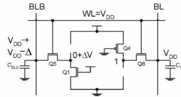
Fig 4: Simplified model of a 6T CMOS SRAM cell during a read operation.
