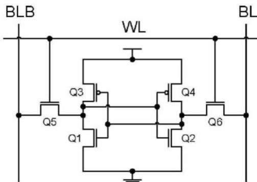
Fig 3: Six-transistor (6T) CMOS SRAM cell.
