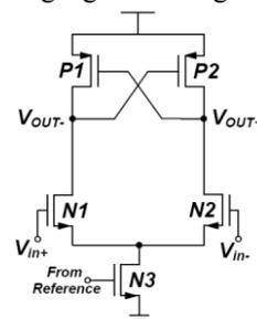
Fig.10 Cross-couple PMOS delay stage with tail current control
