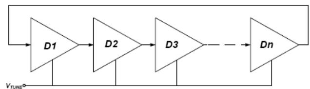
Fig.5 Single-end signal ring VCO
