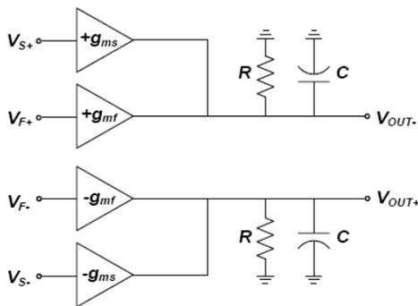
Fig.16 First order model of the delay cell
