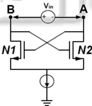
Fig.3 Negative resistor
