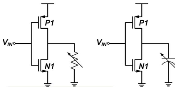
Fig.6 Resistor and capacitor load controlled delay cell
