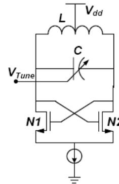
Fig.4 Simple LC resonant VCO
