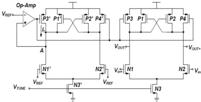
Fig.11 Delay stage with replica bias
