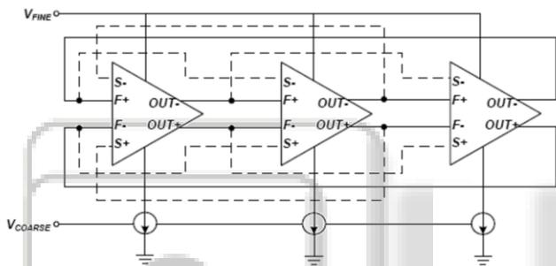
Fig.14 stage multi-loop VCO with first loop (solid line) and second loop (dash line)
