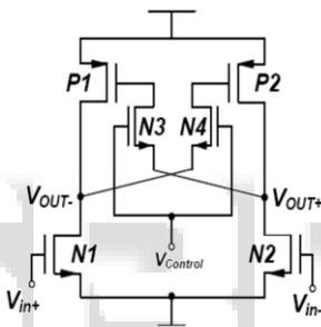
Fig.9 Cross-couple PMOS delay stage with 2 transistors control
