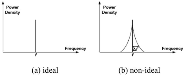
Fig.2 The power density of VCO: (a) ideal and (b) non-ideal
