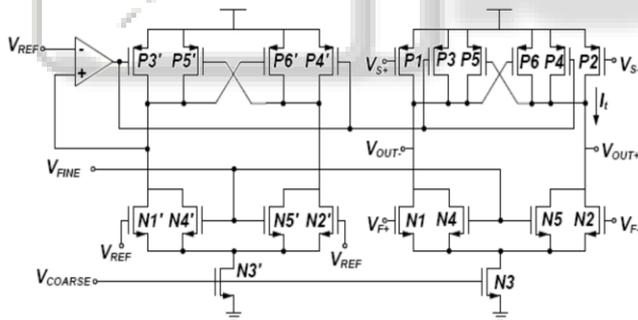
Fig.15 Proposed multi-pass loop delay stage with fine/coarse control
