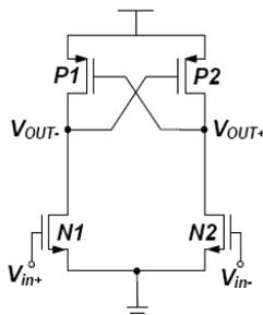
Fig.8 Cross-couple PMOS Delay Stage
