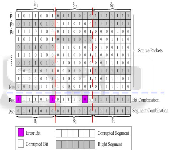
Fig.1. Comparison of Bit Majority, Vote-Based and Segment-Based Packet Combination in the destination.
