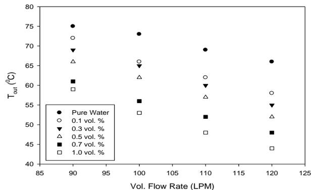
Fig. 7 Comparison of the radiator cooling performance when using nanofluid and pure water
