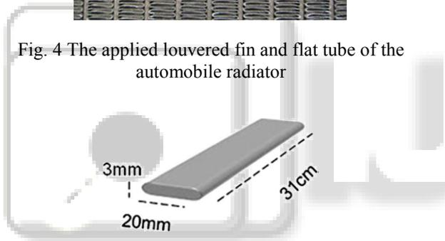
Fig. 5 Schematic and dimensions of the radiator flat tube
