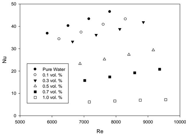
Fig. 8 Nu number variations of nanofluids at different concentrations as a function of Re number ( $T_{in} = 80^{\circ}C$ )
