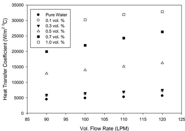
Fig. 9 Experimental heat transfer coefficient of nanofluid at different Vol. Flow Rate
