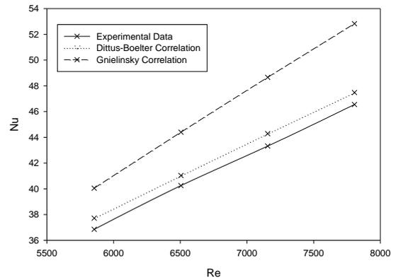
Fig. 6 Experimental results for pure water in comparison with the existing correlations.
