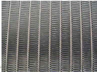
Fig. 4 The applied louvered fin and flat tube of the automobile radiator
