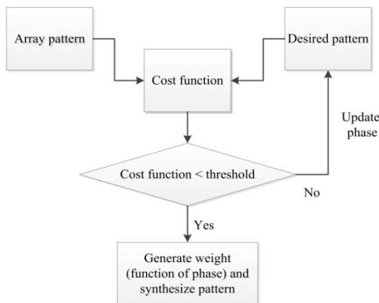
Fig. 1 auxiliary phase algorithm (APA) flow chart.
