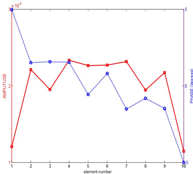
Fig. 4 corresponding excitation to each antenna element.
