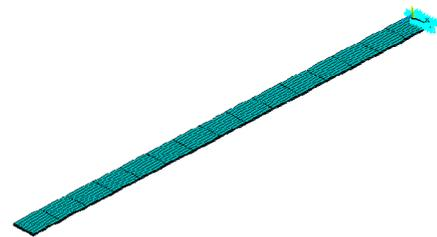
Fig.9: FEA Mesh Model of Cantilever beam
