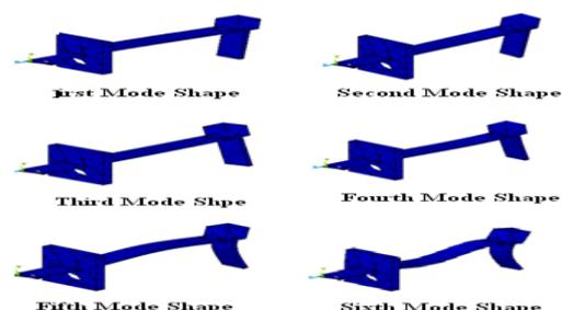
Fig. 7: Mode Shape of absorber for first six natural frequencies at 0.4 L
