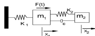
Fig.1: Primary system and absorber schematic
