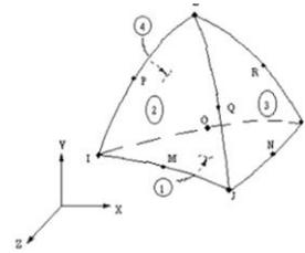
Fig.6: Solid92 3-D-Node tetrahedral structural solid
