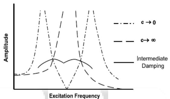
Fig.3: Theoretical response for different amounts of damping
