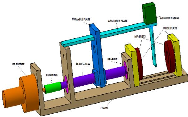
Fig.4: Variable stiffness and variable damping Vibration Absorber
