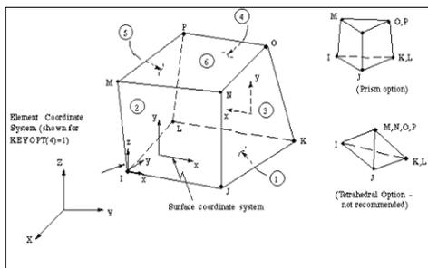
Fig.8 Solid 45 –structural solid
