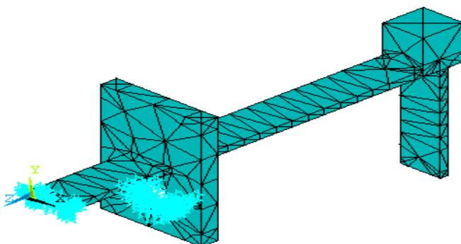
Fig. 5: FEA model of Absorber
