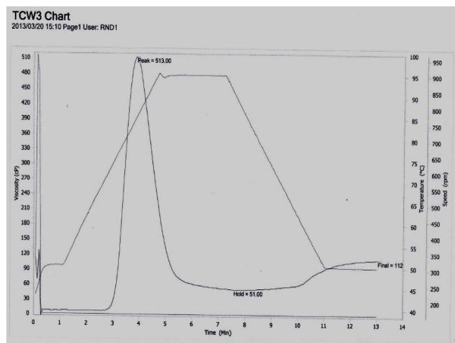
Fig 4. RVA Viscograph of 12% w/w Esterified Starch paste
