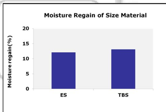
Fig 3. Moisture Regain of Sized Material (TBS-Thin Boiling Starch)
