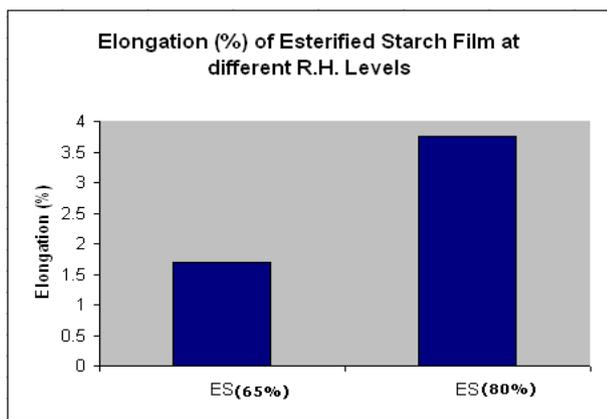
Fig 2. Elongation(%) of ES film at different R.H. levels
