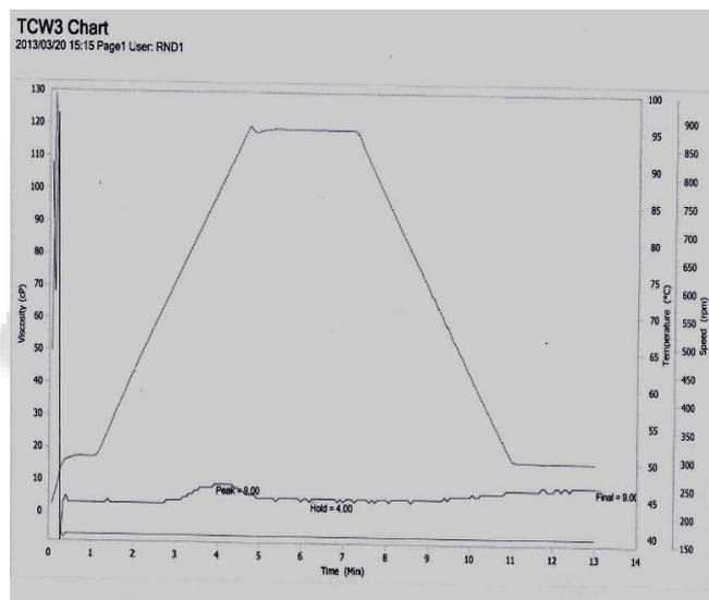
Fig 5. RVA Viscograph – 12% w/w Thin boiling starch paste.
