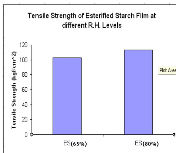
Fig 1. Tensile Strength of ES film at different R.H. levels
