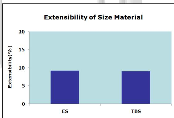
Fig 7. Extensibility of ES and TBS size material samples.
