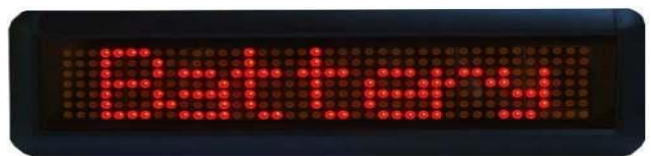
Figure.1: A 5*7 LED electronic Display
