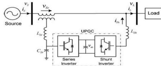
Fig. 1: Unified power quality conditioner (UPQC) system model
