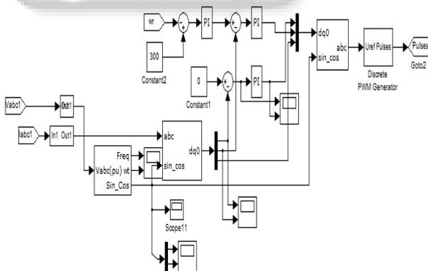
Fig. 3: RSC developed in MATLAB/SIMULINK
