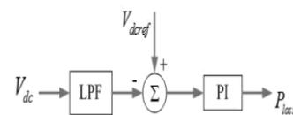
Fig. 6: DC Link Voltage Control Block Diagram.
