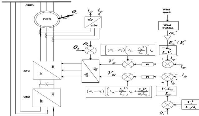
Fig. 2: Vector Control diagram of DFIG
