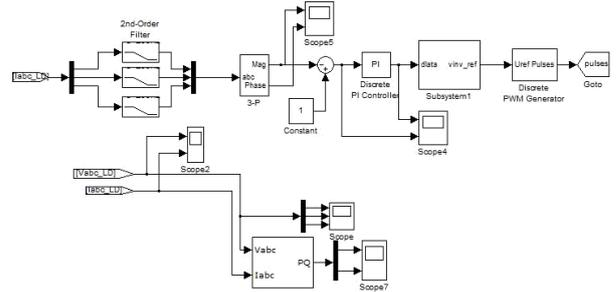
Fig 4: GSC developed in MATLAB/SIMULINK
