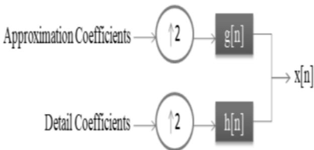
Fig. 5: Block Diagram Of 1-Level IDWT [7]
