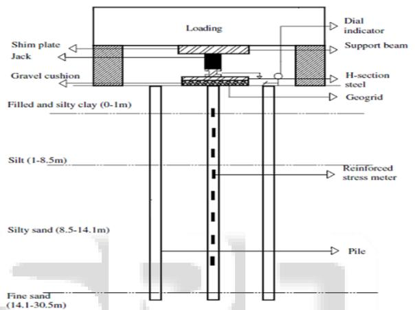
Fig. 4: Layout of test equipment for the static load tests
