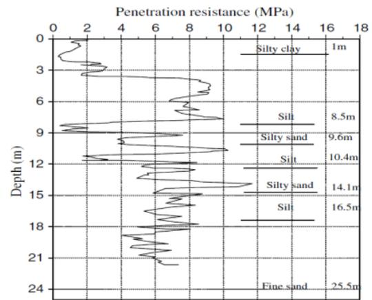
Fig. 3: Result of CPT test for the test site
