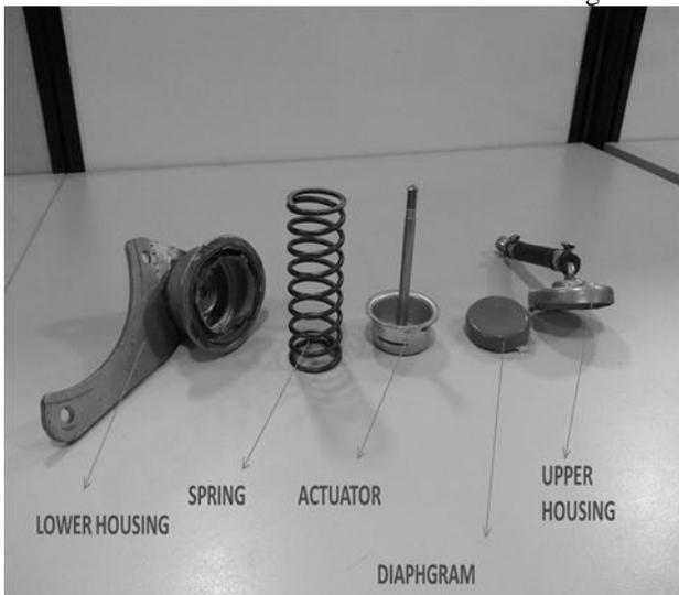
Fig. 6: Dismantled view of the Pneumatic Actuator
