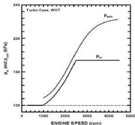
Fig. 3: engine speed vs. inlet and exhaust pressure
