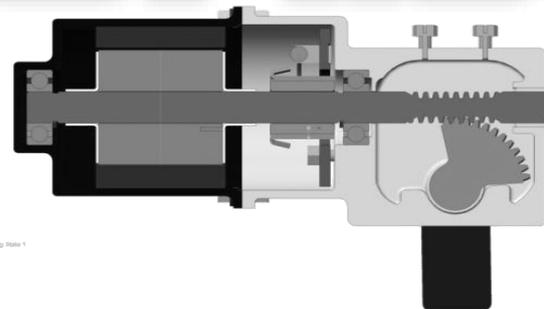
Fig. 13: cut sectional view of actuator
