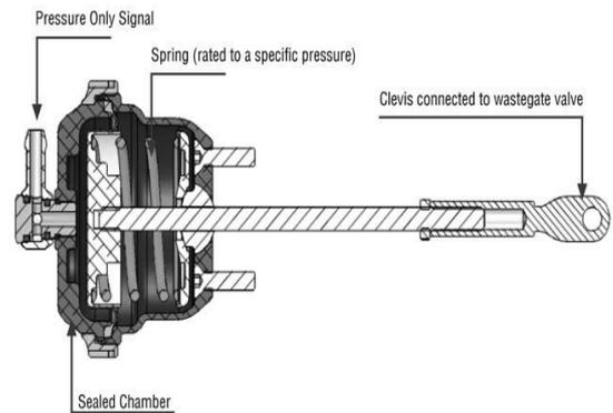
Fig. 4: Pneumatic Actuator
