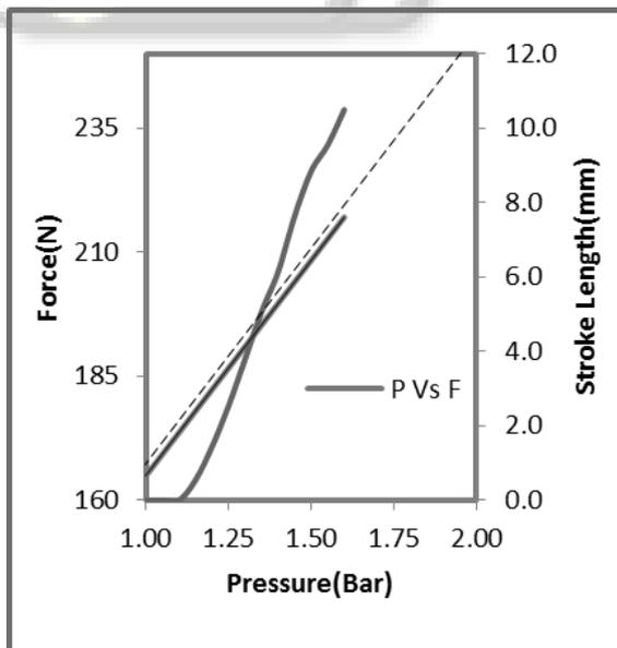
Fig. 7: Graph for pressure Vs. force and stroke Length
