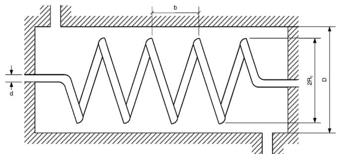
Fig. 3: Schematic view of a typical shell and coiled tube heat exchanger [3]
