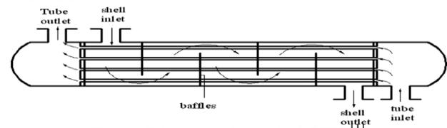
Fig. 1: Diagram of a typical STH
