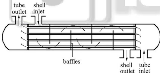
Fig 2: Diagram of a typical shell and tube heat exchanger [2]
