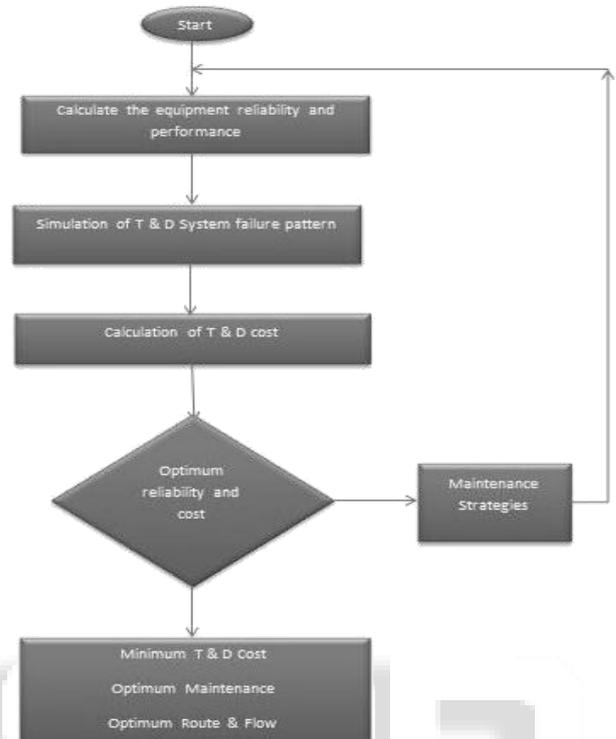
Fig. 3: Flow chart of Intelligent Grid Management System
